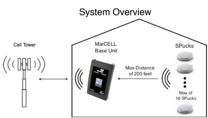
When a Water SPuck detects the presence of water, it wirelessly sends a signal to a MarCELL unit up to 250 feet away. This MarCELL unit then sends a cellular signal to a nearby cell tower which relays it to our servers. Whatever alerts you have chosen on the website (phone call, text message and/or e-mail) are immediately carried out.
